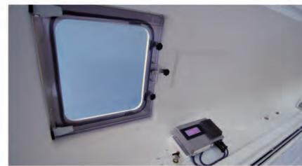
To ensure that users can get out of the capsule during an emergency, the capsule's window can be opened and shut from the inside.
