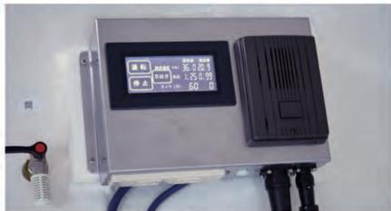
There is also a touch panel monitor on the inside of the oxygen capsule, which displays relevant info such as air pressure level, oxygen level, and remaining treatment time. Users can reduce the air pressure while inside the capsule and perform other adjustments.
