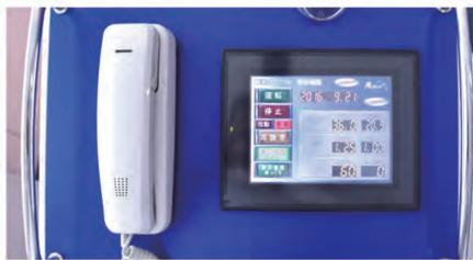
The oxygen capsule has a simple-to-operate LCD touch panel controller. The controller can be used to precision-tune the interior air pressure level by increments of .01 atm, and the automatic controller maintains a pleasant and safe environment inside the capsule.
